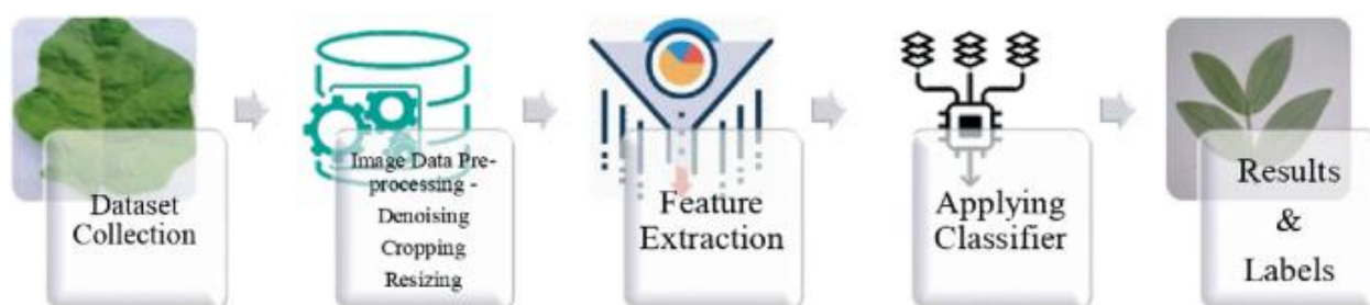
Figure 2. Classification of vegetable leaves using image processing flow chart
