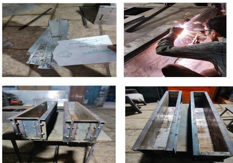
Figure No. 5.4 : Fabrication Of Reinforcement Formwork
