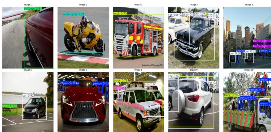
Figure 4.2: Vehicle Detection Output Using Trained YOLOv8 Model
